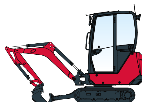
Configuration lame longue / bras long
