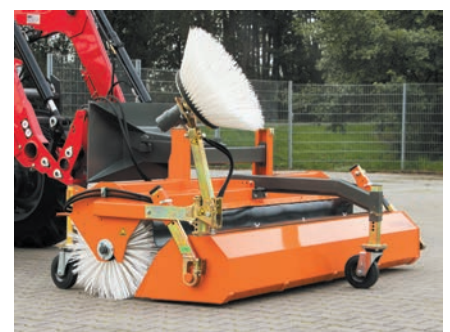
bema 25, collection container with 3rd support wheel
