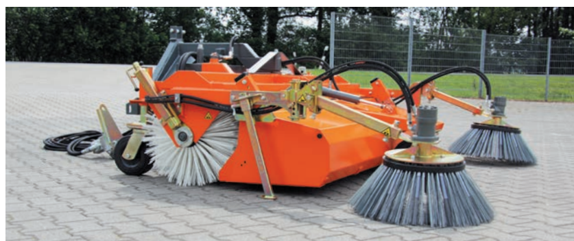
bema 25 Dual with two rotary side brushes for weed removal
